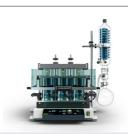
Our SyncorePlus parallel evaporation instrument comes in two configurations; the SyncorePlus Analyst "Pre-Analytical" and the SyncorePlus Polyvap "Throughput".
